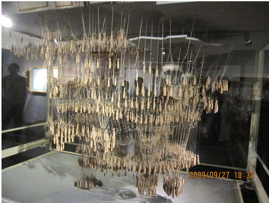
Sand bag model to find the natural shape (minimum bending moment)
